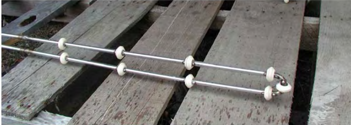
Figure 6. Proprietary TerraTherm Heater Element used Inside the Walls and Floor of each of the Treatment Cells. Covered by one or more of the following: U.S. Patent Nos. 5,190,405, 5,318,116, 6,485,232 and 6,632,047. International patents include EPC 1272290.
